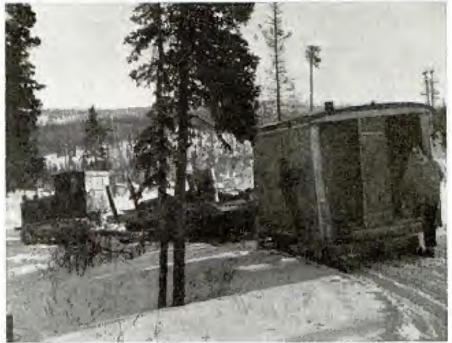
Crawling Diesels haul the "snow trains" laden with supplies. Usually there is a "caboose" serving as cookshed and dormitory
